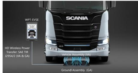
SAE J2954/2 (TM) SAE International Wireless Power Transfer Rendering. Image of Truck Courtesy of Scania.
