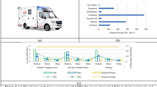
**Figure 1.** (a) The electric ambulance equipped with VIPV, (b) energy demand of ICU medical equipment, and (c) minimum daily energy production in July and December under various parameters and locations.
